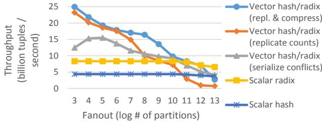
Figure 11: Radix & hash histogram on Xeon Phi
