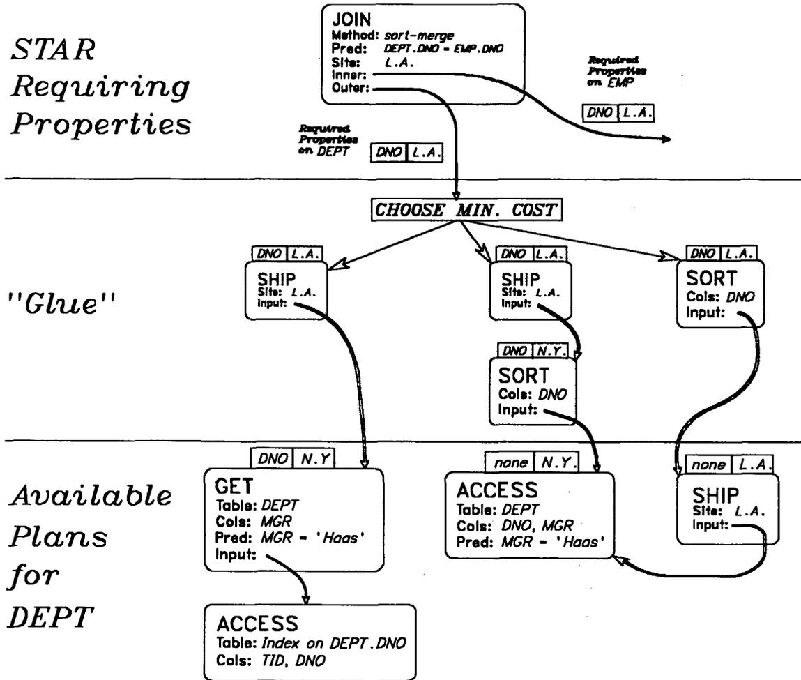
Figure 3: Example of "Glue" mechanism injecting "Glue" operators to match plans to required properties, and choosing the cheapest. Only two properties, order and site, are shown here, as "ears" on top of the top-most LOLEPOP for each plan.
