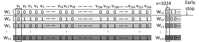
Figure 1: 11-bit column values stored in memory using VBP
