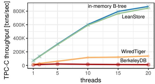
Fig. 8. Multi-threaded, in-memory TPC-C on 10-core system.
