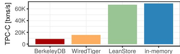
Fig. 1. Single-threaded in-memory TPC-C performance (100 warehouses).
