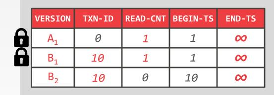
Txns use the tuple's *read-cnt* field as SHARED lock. Use *txn-id* and *read-cnt* together as EXCLUSIVE lock.
