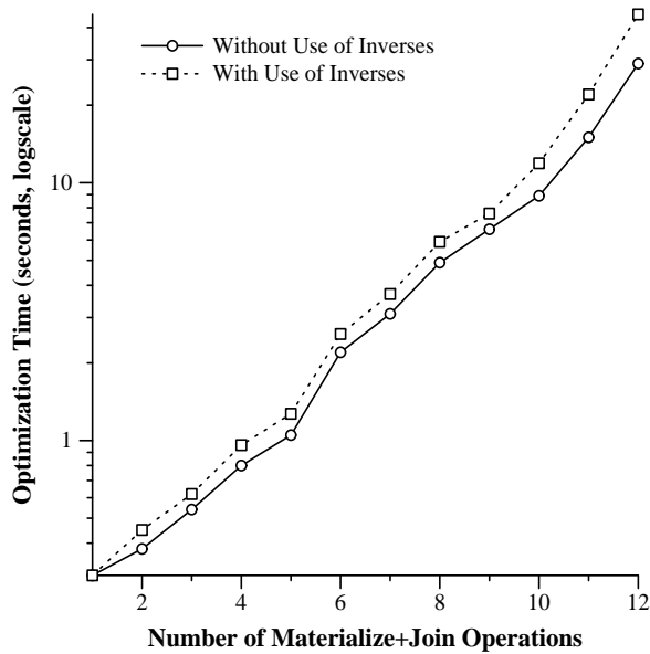
Figure 30: Use of Inverse Links when all references have inverses: Optimization Times (Log-scale)
