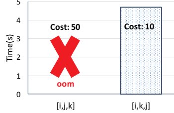
(b) The performance and cost of two attribute orders for sparse matrix multiplication on the nlp240 matrix. The cost 50 order runs out of memory (oom) on a machine with 1TB of RAM.
